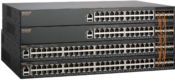
Figure 1: Up to 12 Ruckus ICX 7250 Switches can be stacked together using up to four full-duplex SFP+ h10 Gbps ports for a fully redundant backplane with 480 Gbps of aggregated stacking bandwidth.
